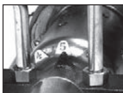
Dial-The-Number Indicator shows number being branded.
